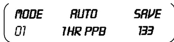
A screenshot of the ozone meter's LCD display. The display is enclosed in a rounded rectangular border and shows three columns of text. The first column reads 'MODE' above '01'. The second column reads 'AUTO' above '1HR PPB'. The third column reads 'SAVE' above '133'.
