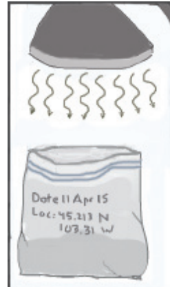
Figure 8, drying soil under a heating lamp
