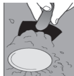
Figure 5, use trowel to dig up sample can
