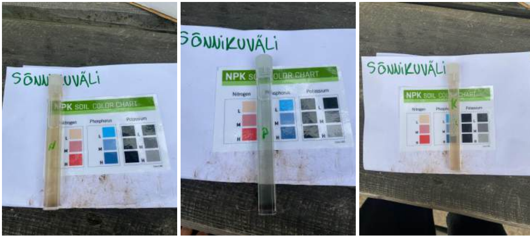
Figure 6. NPK soil testing kit results for the third site - manure-treated field (sõnnikuväli).
