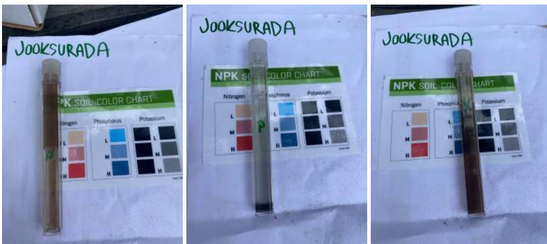
Figure 8. NPK soil testing kit results for the fifth site - running track (jooksurada).
