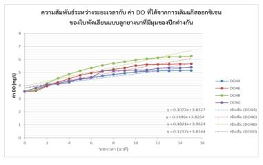
2.2 Study of the number of holes in the wings suitable for oxygenation.
