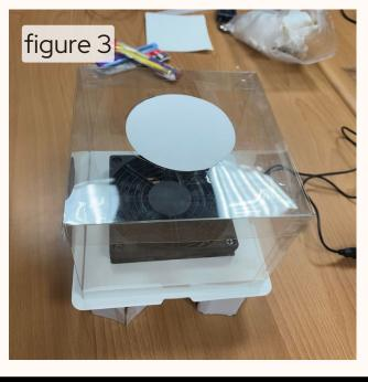
Experimental equipment: exhaust fan, filter paper, cake box, cardboard figure 1 Fixed exhaust fan figure 2 Use cardboard to raise the cake box to allow ventilation figure 3
