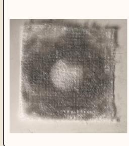
figure.4 The change in the filter paper after measurement (increased by 0.1 grams)2024 Jan 6th~Jan 7th
