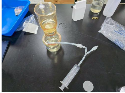
Figure 11. Vacuum filtration device – for microplastic filtration.
