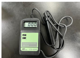
Figure 10. Electrical Conductivity Meter – probe immersed in water to measure EC.
