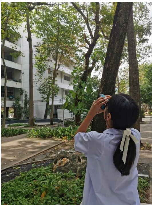
Figure 4: Measuring tree height using a Laser Rangefinder.
