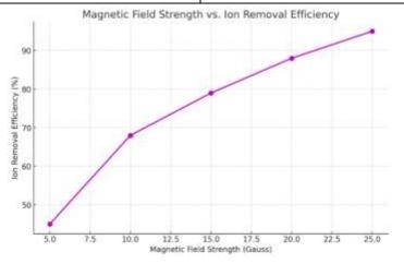
A line chart showing an increase in efficiency as magnetic field strength increases.
