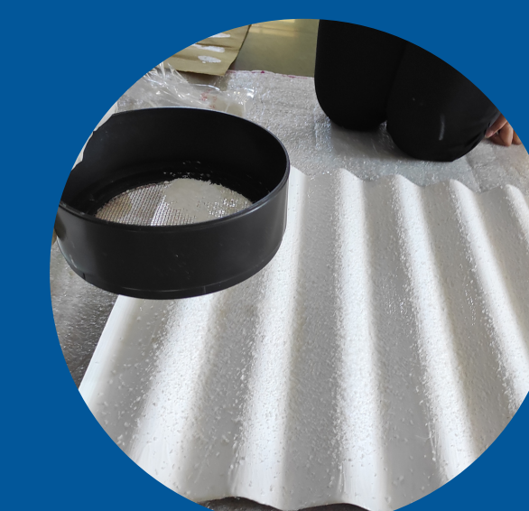
Sprinkling Powdered HDPE
