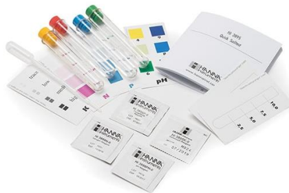
Figure 3.14 Soil fertility test kit with reagents for determining soil N, P, and K values
