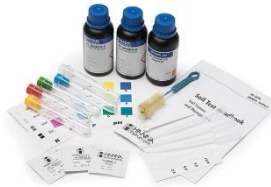
B.3.14 NPK soil test kit
