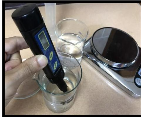
The third experiment: Experiments to measure the drop in water temperature after melting the alum in it.
