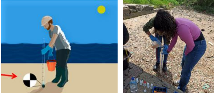
Fig. 1.3: Secchi tube in action.
