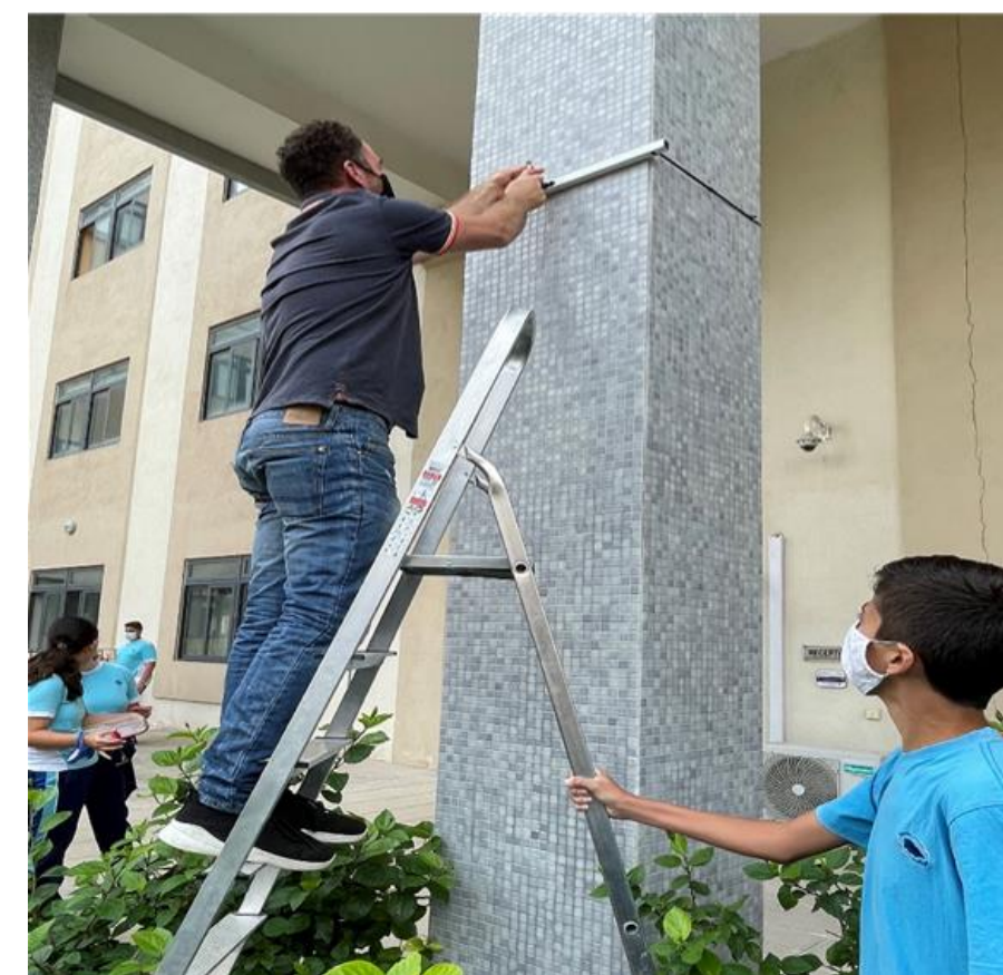
Fig. 3 Setting up one of the diffusion tubes at the main entrance point of Gozo College Secondary School
