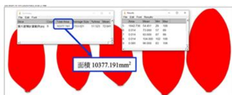
【Figure 7. Calculating the total leaf area using ImageJ】
