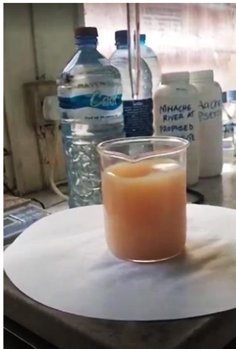
Figure 14: End point of chloride test titration
