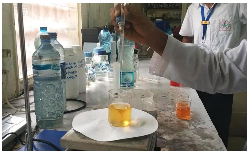
Figure 13: Titration test for Alkalinity
