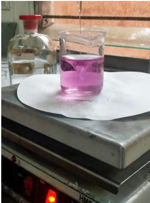
Figure 16: End point of titration test for calcium hardness
