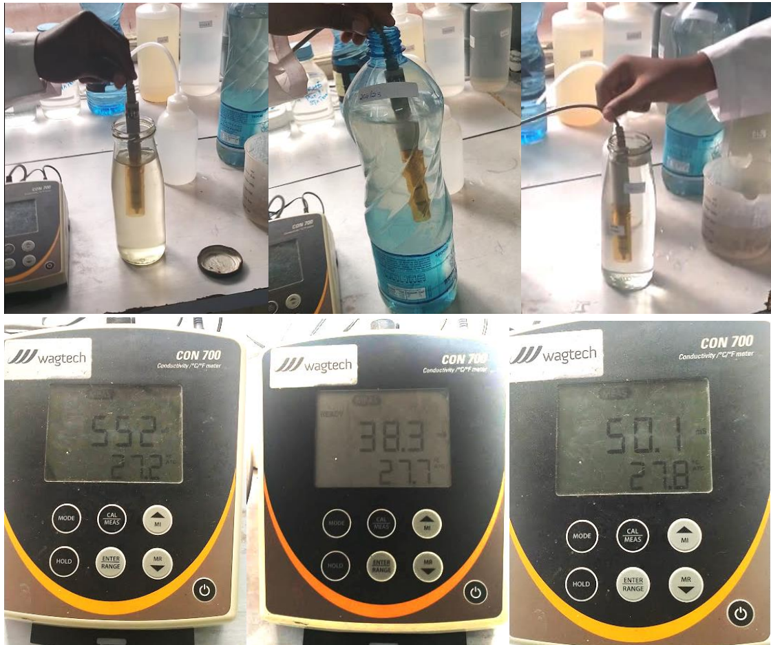
Figure 11: inserted probes and corresponding conductivity readings
