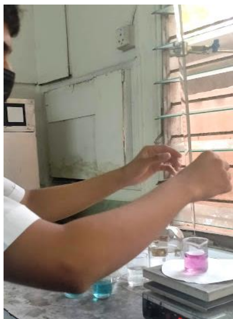
Figure 15: End point of titration test for total hardness
