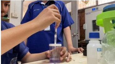
Picture 1 , 2 Measurement of water hardness.
