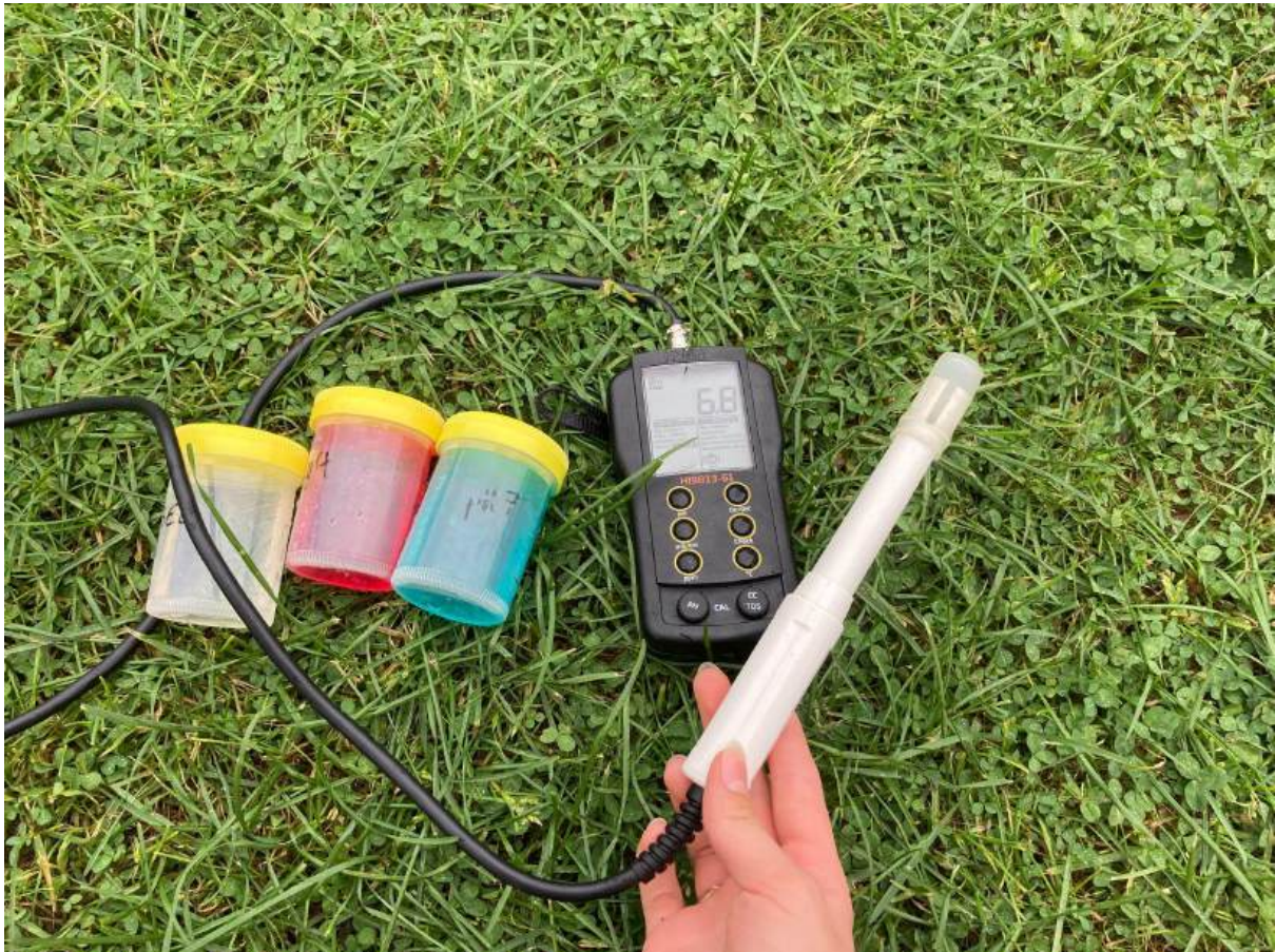
Figure 3. Multimeter and the solutions used to calibrate it (M. Loit)
