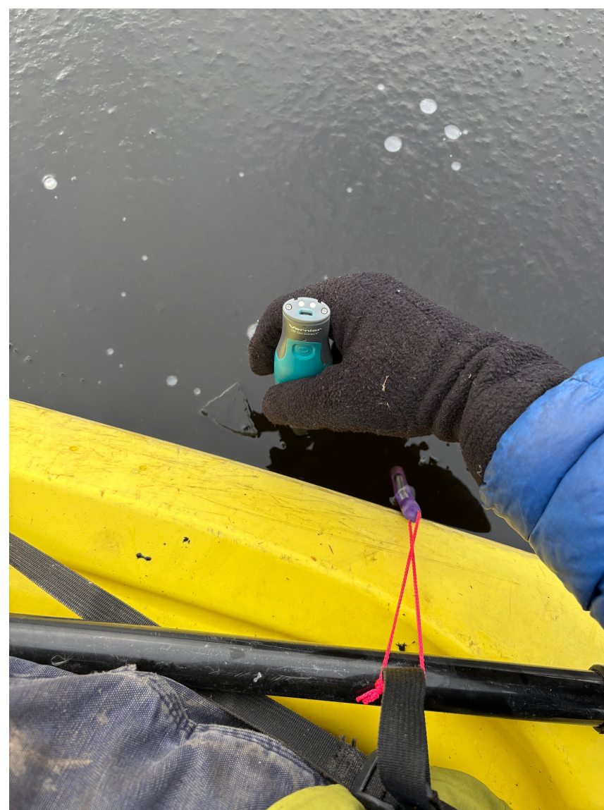
Figure 5. Dissolved oxygen being measured with a probe and water temperature being measured with an alcohol thermometer on 10/19/25 through a thin layer of ice.
