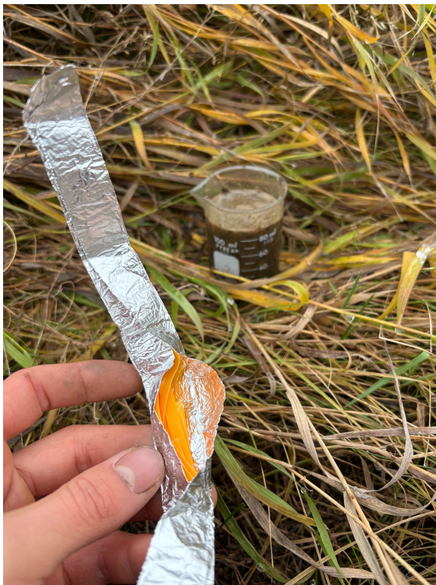
Figure 6. Soil pH being measured from a 1:1 ratio solution with distilled water. pH tape stored in tin foil.
