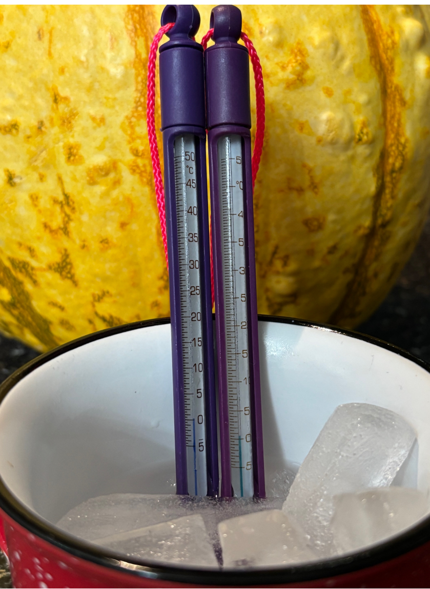
Figure 4. Alcohol thermometers calibrated in ice bath.
