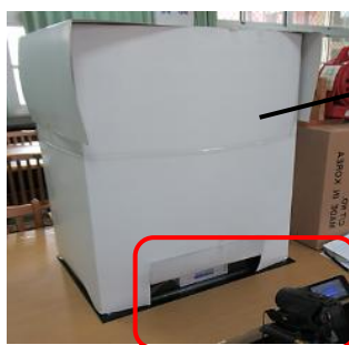
【 Figure 7. Diagram of the respiration experiment with a light-blocking cover installed 】
