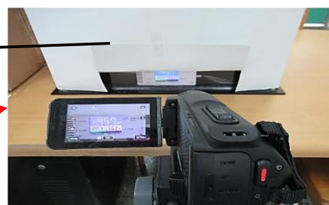
【 Figure 8. Diagram of the light-blocking cover with a side opening at the base for video recording 】
