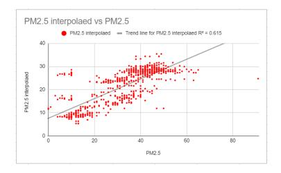
Figure 5D Compare the pm 2.5 value of the AirLink air quality meter and the researcher's air quality measuring device. Dam Ridge area
