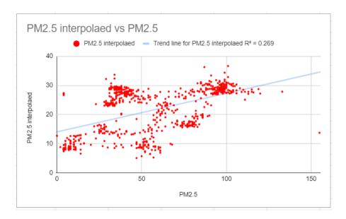
Figure 5E Compare the pm 2.5 value of the AirLink air quality meter and the researcher's air quality measuring device. Parking Lot
