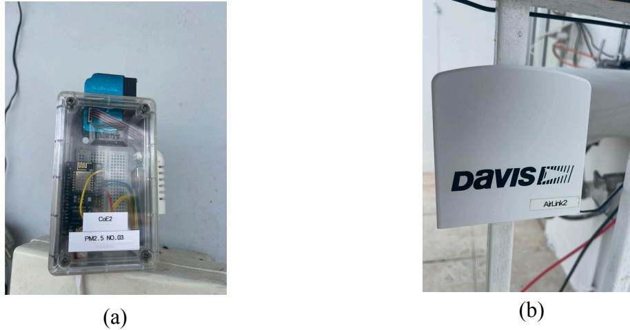
Figure 3. (a) Plantower Laser PM 2.5 dust sensor PMS3003 with IoT and (b) Davis AirLink station installed at one of our study locations.
