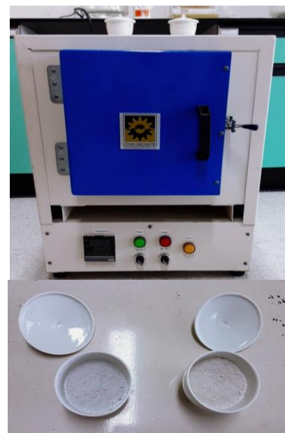
Figure 4. Burning of oyster shell using the furnace.
