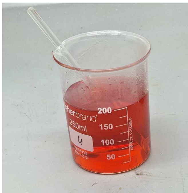
Figure 9: 'Piranha solution' – soil digestion
