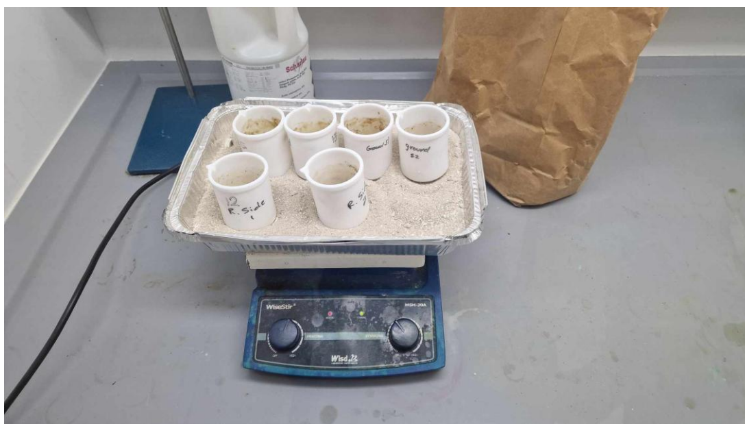
Figure 11: Samples cooling down during soil digestion
