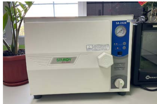
Figure 4. Sterilization of the equipment using the autoclave.
