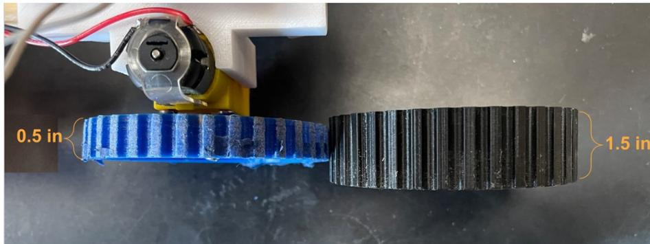
**Figure 8. 3D-printed TerraRover 2 Wheels.** Image above includes the different dimensions of the wheels used during data collection. The researchers independently used computer-aided design (CAD) to model new wheels for the TerraRover 2 with an increase to 1.5 inches. The researchers were aided by Mr. Andy Henry during the modeling process and 3D-print the design at Wayne RESA.
