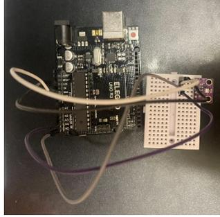
**Figure 5. BME280 Temperature, Humidity, and Barometer Sensor.** Image above displays the BME280 Temperature, Humidity, and Barometer Sensor the researchers used to collect temperature and humidity data. The sensor was placed on a platform connected onto the TerraRover 2, secured by industrial zip-ties. The BME280 Temperature, Humidity, and Barometer Sensor was programmed by the researchers using the Arduino IDE and Arduino programming language.
