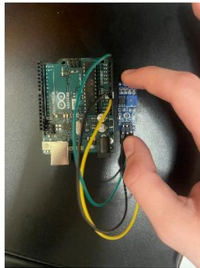
**Figure 6. Photo Resistor Sensor.** Image above displays the Photo Resistor Sensor the researchers used to collect light intensity data. The sensor was placed on a platform connected onto the TerraRover 2, secured by industrial zip-ties. The Photo Resistor Sensor was programmed by researchers using the Arduino IDE and Arduino programming language.
