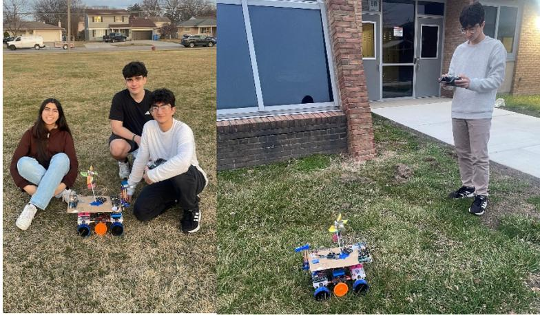
**Figure 9 and Figure 10. TerraRover 2's Use at Crestwood High School.** Images above greatly shows TerraRover 2 at Crestwood. Throughout the research, the TerraRover 2 was being driven to efficiently collect data for light intensity, sound, proximity, temperature, humidity, and pressure.
