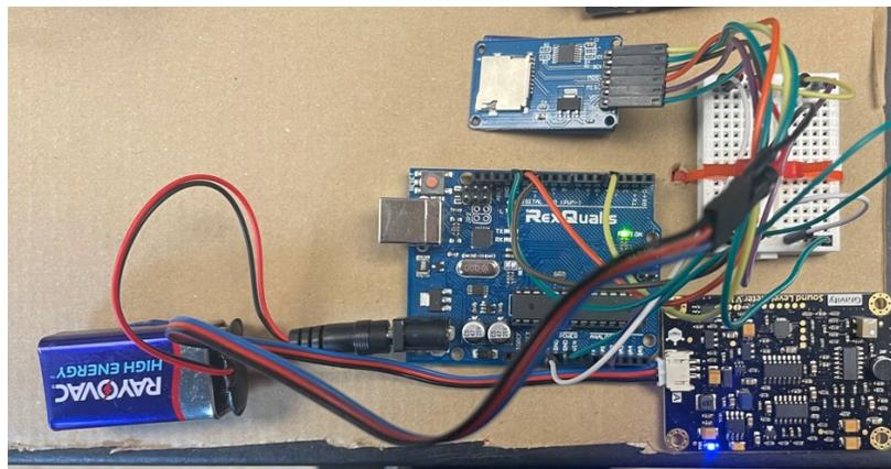
**Figure 4. Sound Sensor.** Image above displays the Sound Sensor the researchers used to collect sound (dBA) data. The sensor was placed on a platform connected onto the TerraRover 2. The sound sensor was programmed by the researchers using the Arduino IDE and Arduino programming language.
