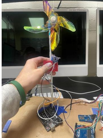
**Figure 3. VCNL4010 Proximity/Light sensor.** Image above displays the Proximity Sensor the researchers used to collect wind speed data. The sensor was placed on the top of the TerraRover 2, secured on an elevated platform. The VCNL4010 Proximity/Light sensor was programmed by the researchers using the Arduino IDE and Arduino programming language.
