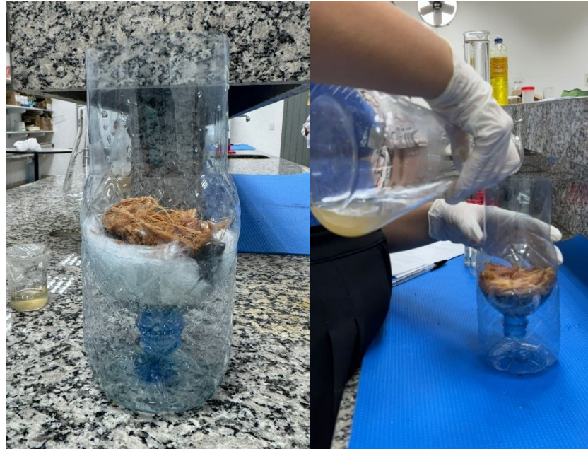
Figure 3 – Representation of the filter prototype used for the filtration of the samples.
