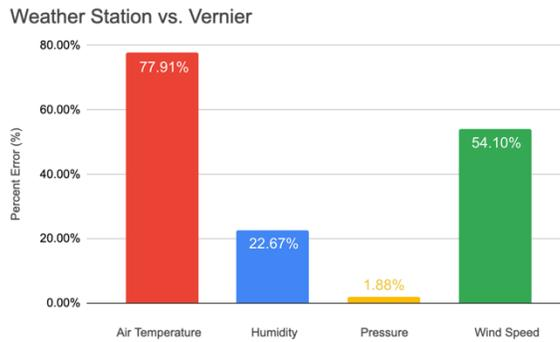
**Figure 16. Weather Network HD CCD Video Camera vs Vernier (Dearborn Heights).** The graph above shows the percentage error of air temperature, humidity, pressure, and wind speed between the Weather Station and the Vernier Go Weather Direct Device in Dearborn Heights, Michigan. Air temperature and wind speed have high percent errors of about 77% and 54%, while humidity has a percent error of approximately 20%. Pressure has the lowest percent error, hardly reaching 2%.
