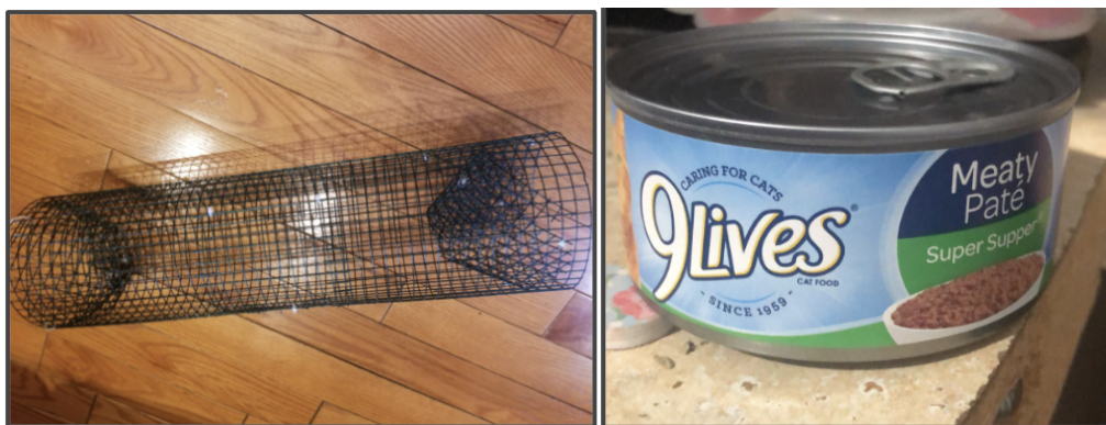
Figure 5-6 Trap Mechanisms. Figure 5 (left) shows one of two traps built for this study. They had been built from mesh wire with the dimensions of .6 meters long and with a diameter of .17 meters. Figure 6 (right) is the bait used which is a can of cat food.
