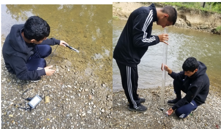
Figure 7-8 Equipment. Figure 7 (left) shows the LabQuest 2 where the optical DO probe and temperature probe can be attached to give the readings. Each probe is dipped into the water and the team reports the results displayed on the LabQuest 2. Figure 8 (right) shows the turbidity tube. The tube gets filled with river water and is drained until the pattern on the bottom of the tube is visible. Then the tube stops being drained and the water level is recorded to give the group the turbidity measure.
