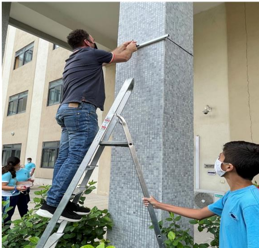
Figure 3: Setting up of one of the diffusion tubes at the main entrance point of Gozo College Secondary School
