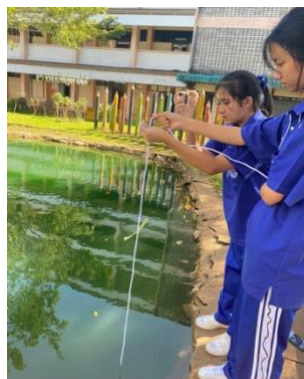
Find the conductivity in water Using a Conductivity meter.
