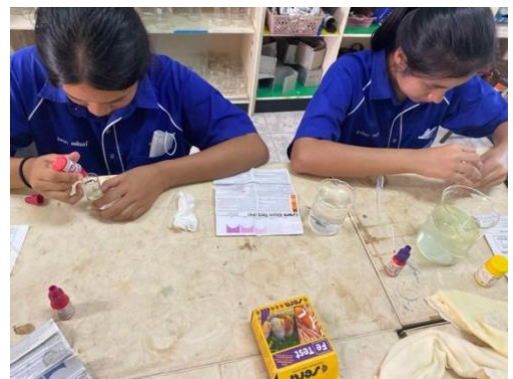
Find the iron and phosphate values using Phosphate Test and iron Test.
