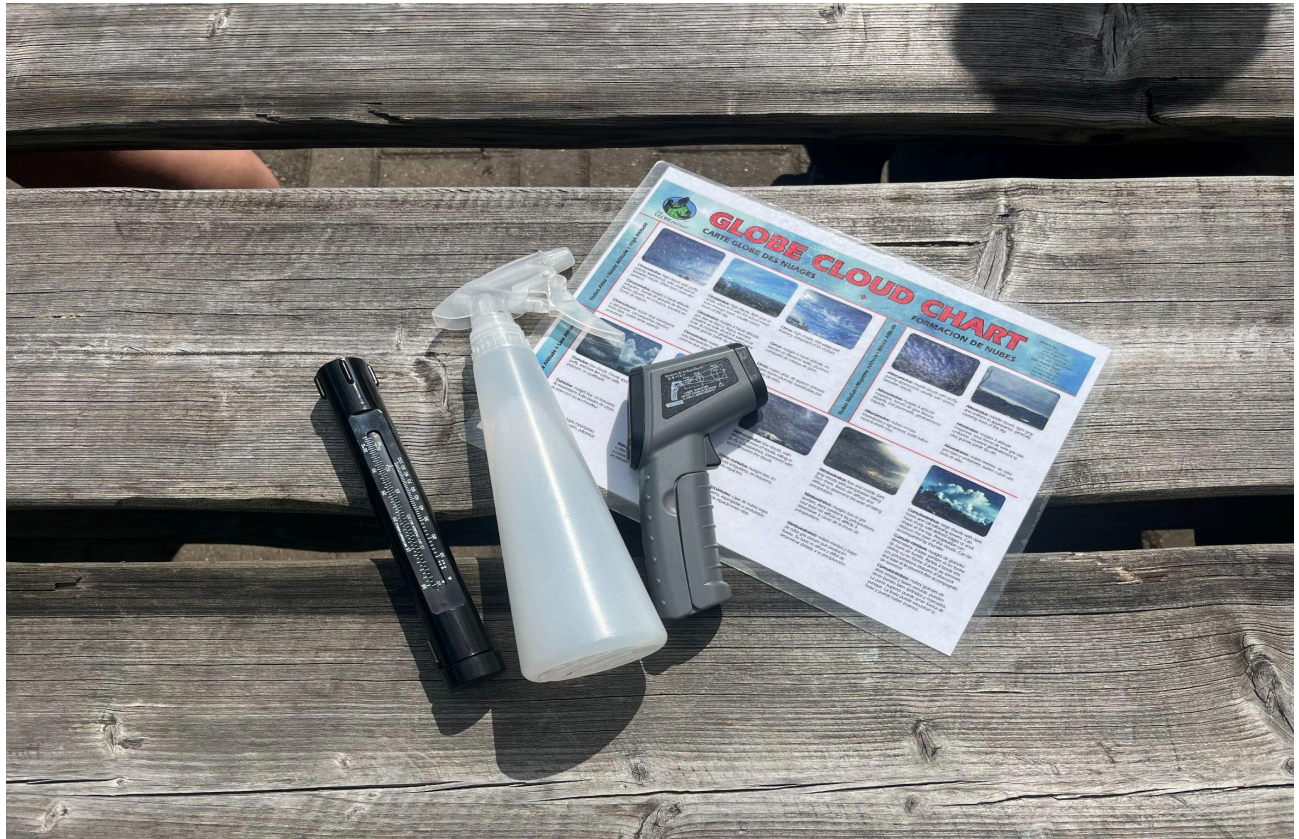
Figure 2. Measurement instruments: sling psychrometer, water bottle for the wet-bulb test, infrared thermometer, cloud chart.
