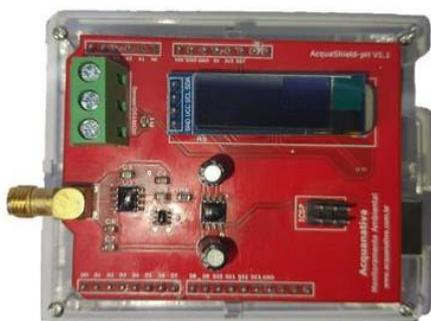
**Figura 8 – Placa Shield pH**
