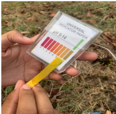
Measure pH using universal indicator paper.
