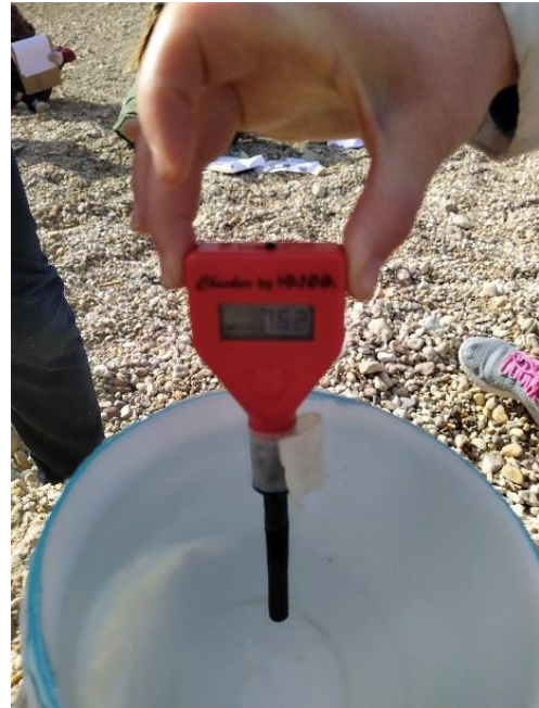
Measuring sea water temperature and pH level using specialised equipment
