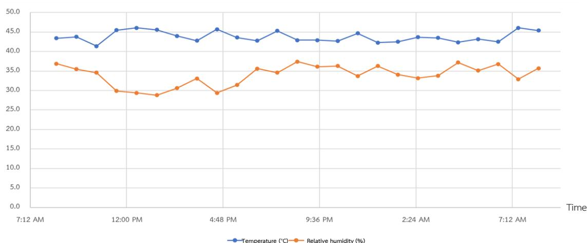
**Figure 8:** Shows the temperature and relative humidity inside the cabinet.
