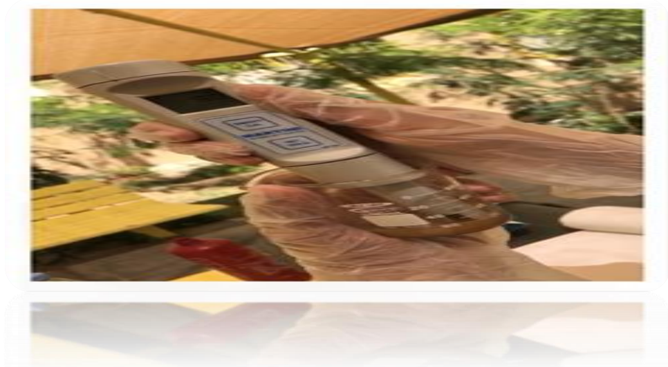
Figure (3) shows ph measurement of the second and third layer = 8
