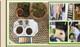
Soil characterization in terms of acidity, bicarbonate, and color, and a comparison between Al-Mattan and Al-Baha soils Figure (6)
