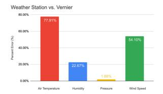
**Figure 16. Weather Network HD CCD Video Camera vs Vernier (Dearborn Heights).** The graph above shows the percentage error of air temperature, humidity, pressure, and wind speed between the Weather Station and the Vernier Go Weather Direct Device in Dearborn Heights, Michigan. Air temperature and wind speed have high percent errors of about 77% and 54%, while humidity has a percent error of approximately 20%. Pressure has the lowest percent error, hardly reaching 2%.
