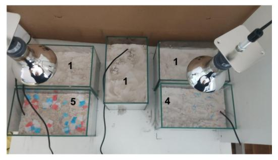
Picture 2. Experimental setup during the research (label 1- control group, label 4- the group with microplastic in the sand, label 5- the group with microplastics in the sand and plastic on the surface)
