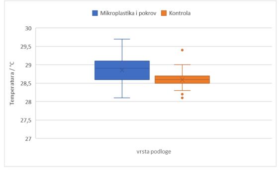
Figure 8. Comparison for soil temperature of sand with microplastic within and microplastic pieces on top and control group; the box shows the standard deviations, the horizontal line presents average value, and the vertical line the minimum and maximum values, with a dot display of extreme values.
