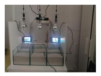
Picture 1. Experimental setup during the process of system calibration to the same input of heat
