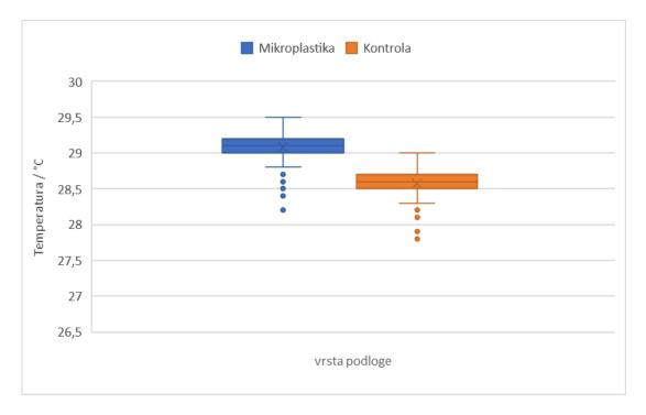
Figure 7. Comparison of sand temperature with microplastic mixture and control group; the box shows the standard deviations, the horizontal line presents the average value, and the vertical line the minimum and maximum values, with a dot display of extreme values.
