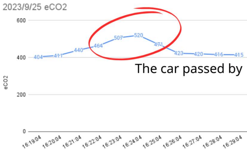
(Figure3. Changes in carbon dioxide concentration when a car passes by)
