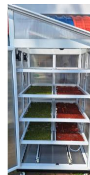
Figure 6-7: Cabinet's draft Figure 8: Shows the pepper drying cabinet, while drying pepper
