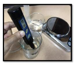
The third experiment: Experiments to measure the drop in water temperature after melting the alum in it.
