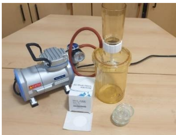
Figure 3 Vacuum filtration equipment
