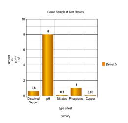
Now this sample came from further out of the main city, almost the last customer on the city line. The phosphates are lower, but there is still copper and nitrates present in the water. Lead was also confirmed via a different test. Look at the pH level. It is basic, which is another type of corrosion. Basic leaves corroded `stuff' behind, in your water, while acidic 'eats it away'. This sample came from Newport area.
