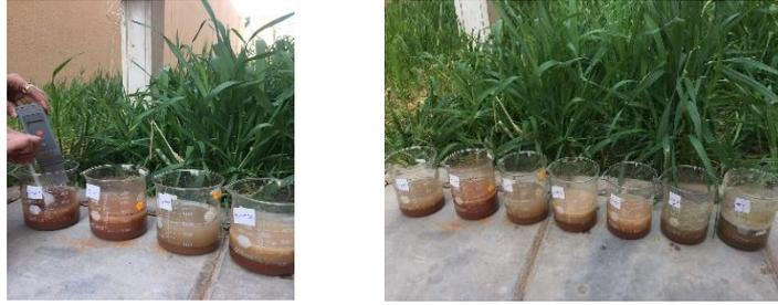
Figure 8: The experience of pH measurement of soil (from experiments we conclude that the soil types are acidic or alkaline (figure 9).
