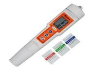
Figure (1) Digital soil pH meter
