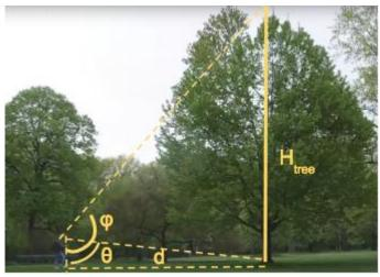
**Figure 4.** Geometry of tree height measurement. Schematic of tree height observation made using the Trees tool in the GLOBE Observer mobile app. 0 degrees is straight down, 90 degrees at the horizon, 180 degrees is straight up.
