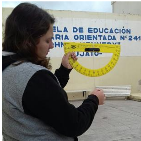
Figure 5: Student assembling the clinometer and testing it on the site
