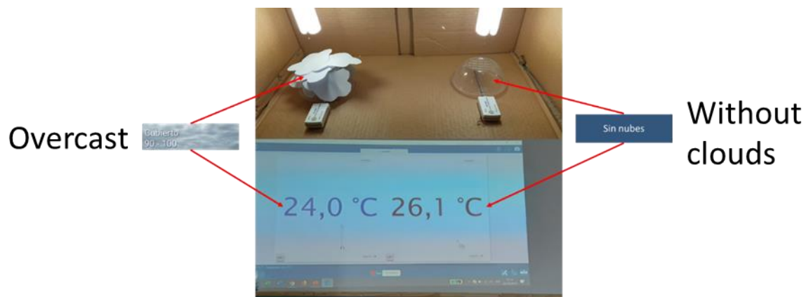
Fig. 8. Experiment to simulate the effect of clouds on the temperature of the atmosphere. (Smith, & Owens, 2003)
