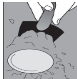
Figure 5, use trowel to dig up sample can
