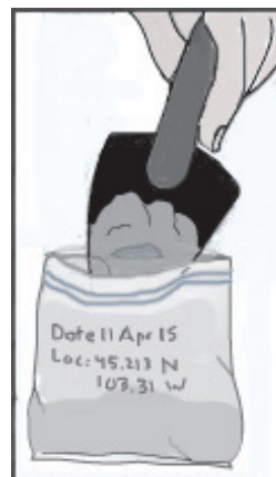
Figure 3, placing soil in zip lock bag
