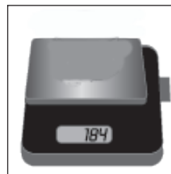
Figure 7, determine wet mass of soil sample and bag
