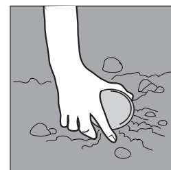
Figure 4, pushing sample can into soil
